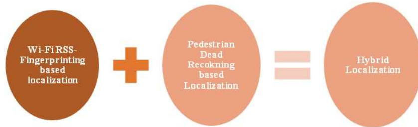
Figure 6. Proposed hybrid IP system.
