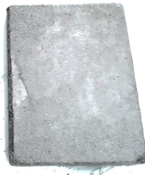
Figure 3. The graphite-based electrode used in the ionizer.
