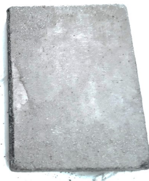
Figure 3. The graphite-based electrode used in the ionizer.
